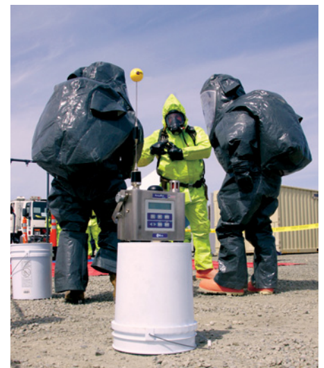
A HazMat Team utilizes the strategically-placed AreaRAE to provide real-time detector to establish a perimeter and monitor PID, LEL and VOC readings.
