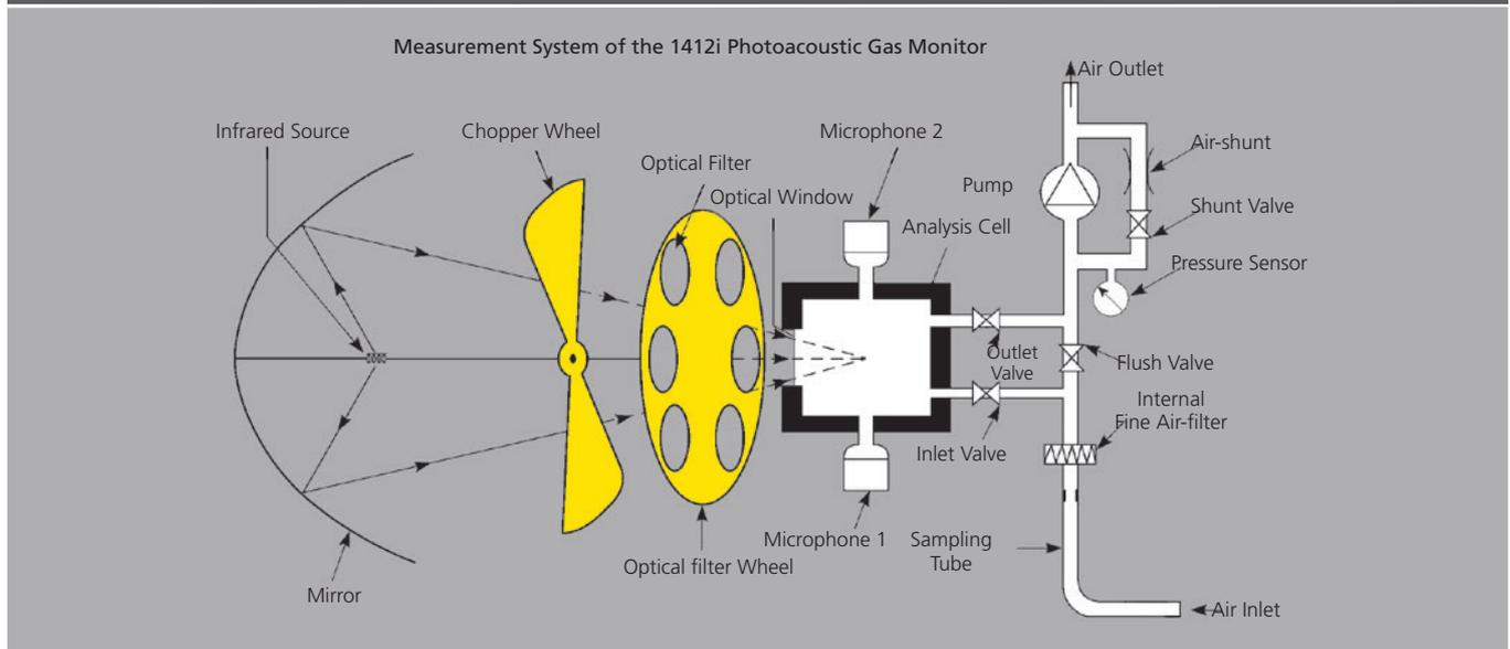
1. The pump draws air from the sampling point through the air filter to flush out the "old" air in the measurement system and replace it with a "new" air sample. The pressure sensor is used to check that the pump sequence is elapsed successfully and to measure the actual air pressure.
